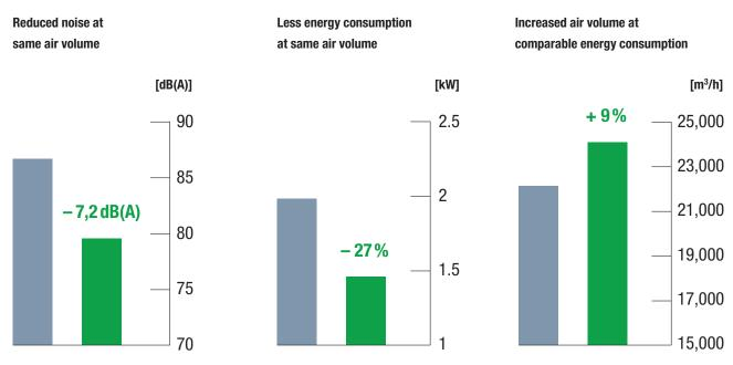
Comparison figures measured in application, each with EC fans of size 800.
